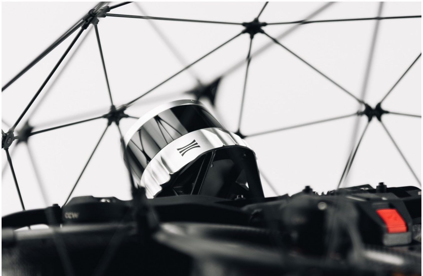
The Elios 3 with the Surveying Payload mounted
