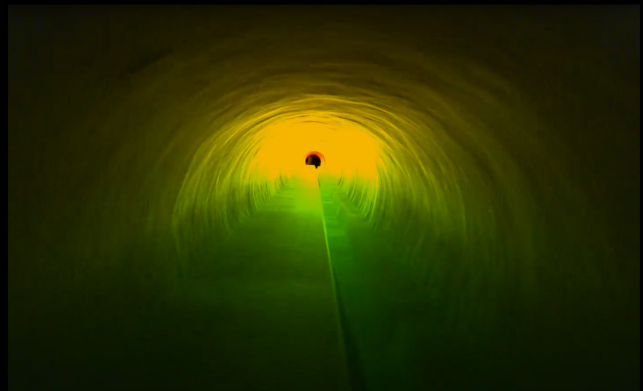
3D model in a challenging symmetrical environments; >2m diameter with light geometric features/texture in long straight parts (>30-50m)
