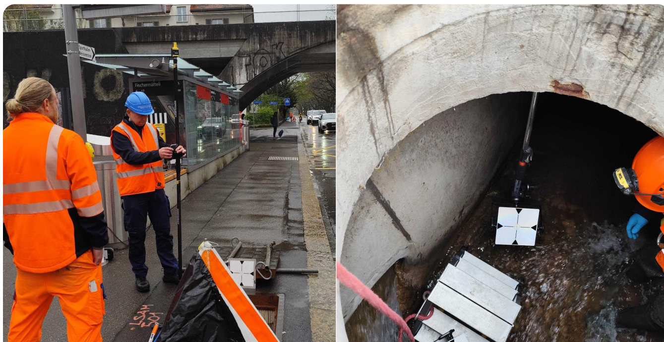
The target positions on site are placed at different angles as georeferencing points
