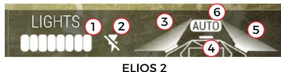
The LED lights status displays the power level of the lighting system and which panels are lit on ELIOS 2.
