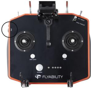
The tilt of the payload can be controlled with the rotary lever on the left side of the remote control. For clarity, the payload tilt angle is displayed on the left side of the tablet's screen during flight.
