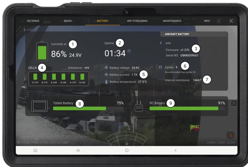
Figure 6.7: ELIOS 3 Battery Panel
