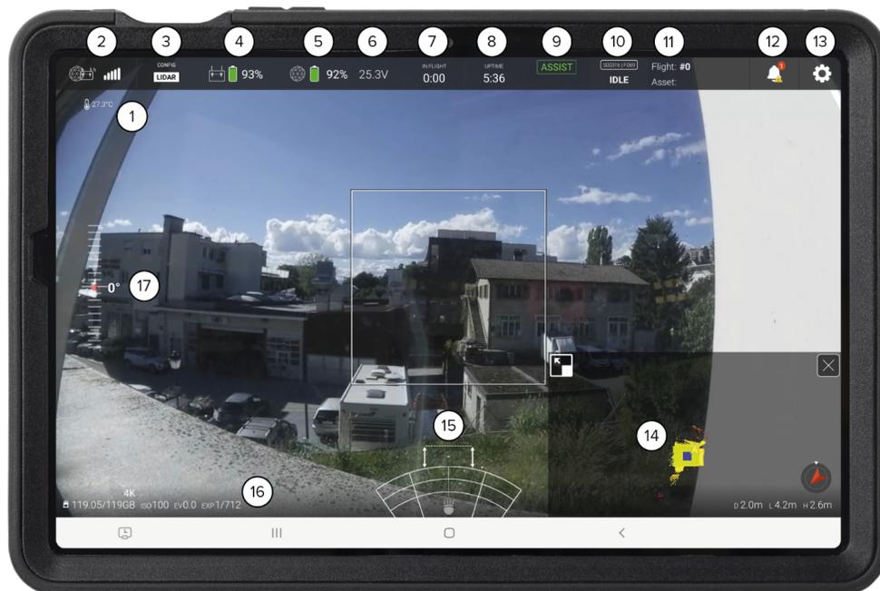
Figure 6.4: ELIOS 3 cockpit
