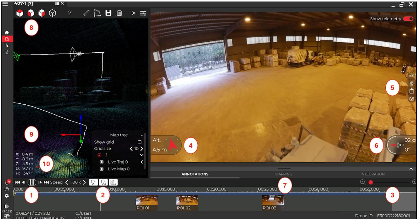
Figure 9: Inspector 4 Flight Screen
