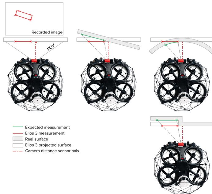
Figure 11.4 Inspector 4 Add Measurement
