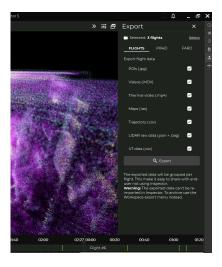
You will get a .CSV file containing the following information: flight name, POI name, thickness, calibration speed, X, Y, and Z coordinates, payload serial number, and probe serial number.
