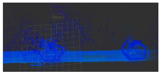
**Previous release** : After flying back and forth in this tunnel, there is a drift of 14m, resulting in the hexagonal structure appearing twice in the map.
