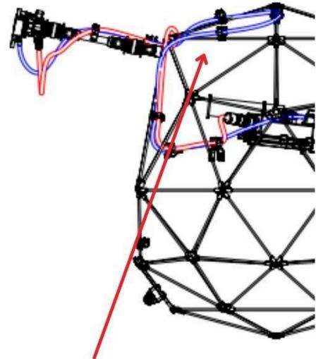
It is CRITICAL that cables are placed outside the cage
