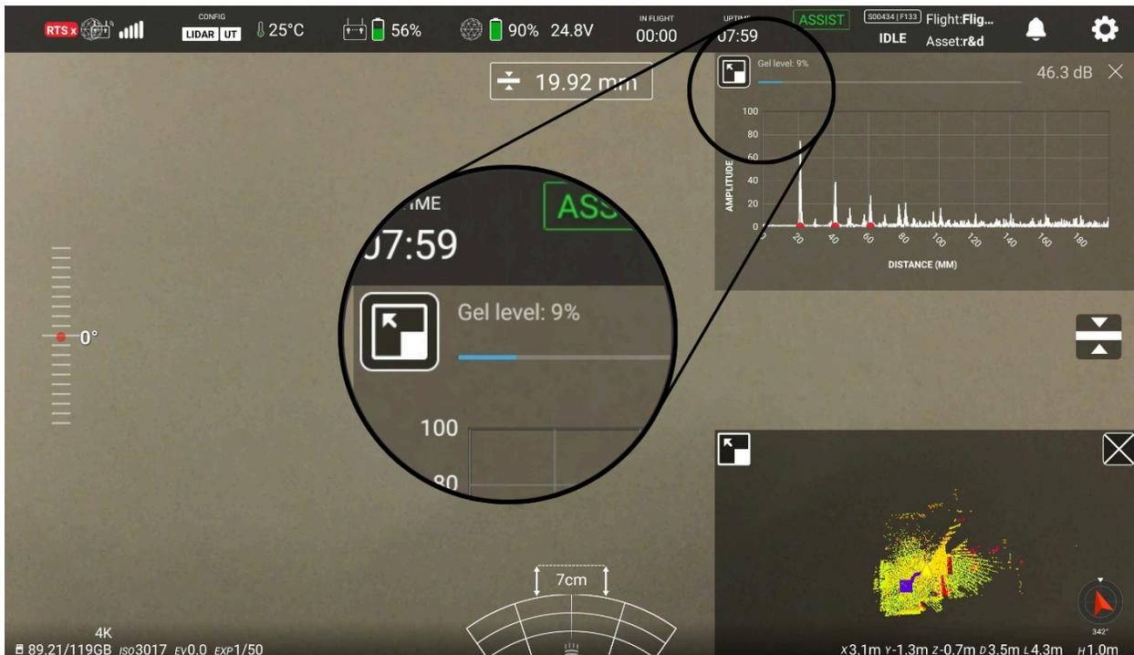
We also suggest having several smart syringes filled with couplant before starting an inspection. In this way, you will not have to refill them manually on the field but rather you will be able to quickly swap the syringe before a flight, reducing inspection time and avoiding the issue of being out of couplant.
